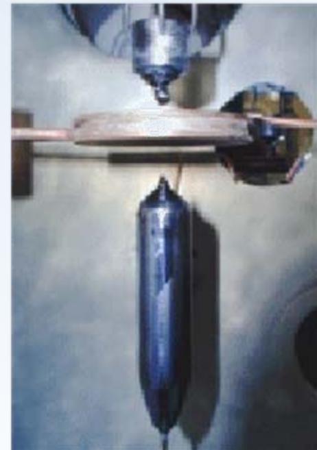
Fig. 1c. Finished FZ ingot
