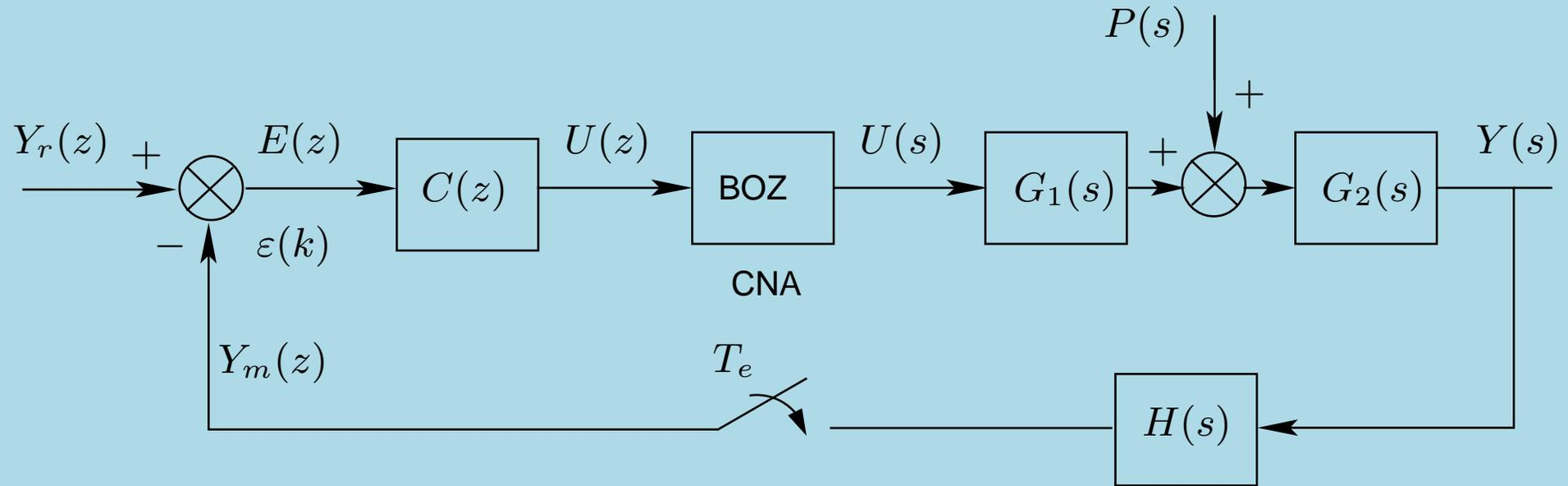
$$Y(z) = \frac{C(z) (1 - z^{-1}) \mathcal{Z} \left\{ \frac{G_1(s)G_2(s)}{s} \right\}}{1 + F_{BO}(z)} Y_r(z) + \frac{\mathcal{Z} \{ G_2(s)P(s) \}}{1 + F_{BO}(z)}$$
